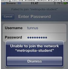
To join a new network, it is best to first disconnect from the current network (Forget this Network) and then join the new network. If you are too quick, you will get the same error message. Wait a moment and try again.
