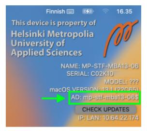
If IP:LAN shows a bunch of question marks then computer's network is not connected properly and login will not be successful.
